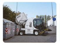
The multi-level dumping system provides emptying of the hopper at heights from 80 to 160 cm on RS 850 and RS 1300
