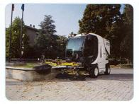
The RS 1300 and RS 850 have an option to be fitted with a third brush that can be elevated to clean at varying heights.
