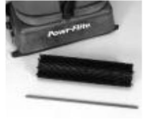
Withdraw shaft completely.
