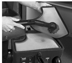
**Note:** You may want to have several extra filters on board the Liberator so you do not have to leave the area to clean the filters. Just replace the dirty filters with clean filters and continue cleaning. Then you can clean the dirty filters later.
