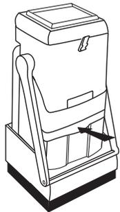
Push hopper firmly into hopper guides to insure a snug seal.
