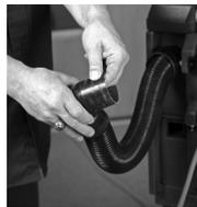
2. Check the vacuum shoe between the cleaning brushes on the underside of the Freestyle for buildup. With a tank vacuum, remove any material clogging the shoe.
