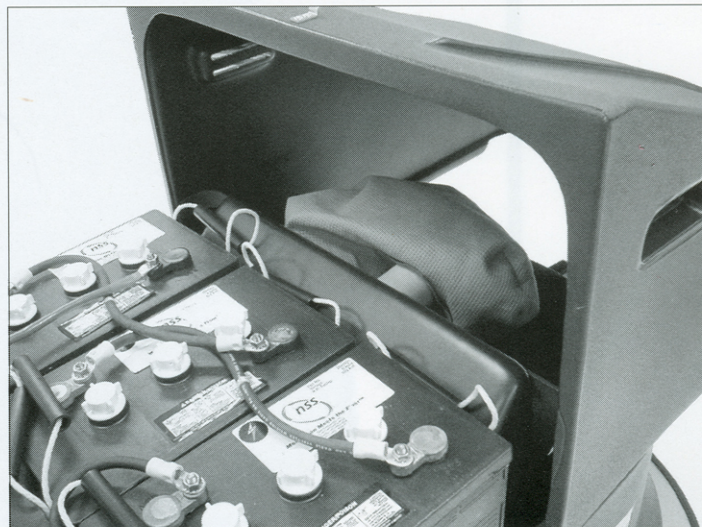
The Vac-Trac™ Dust Control System collects pad dust in a filter bag at the front of the machine (under the sliding battery compartment lid).
