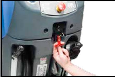
Located to the rear of the machine is the charger inhibit plug.
