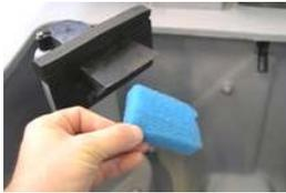
Check the detergent output filter is undamaged and clean. Always remember to close the valve upstream of the filter before checking.
