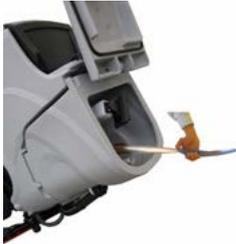
Check the suction filter is undamaged and clean.
