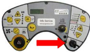
3. Press the brush button to enable brush and suction motor operation. Hold the button down for at least five seconds to select the operating mode MICROFIBRE / BRUSH-PAD.
